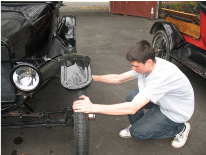
Check out the king pins with a good yank or two.
